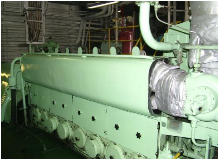
Pervomaisk Dieselmash, 4 stroke, 8 cylinder, Model 8CHN25/34-3, constructed in 1986 500kW engine
